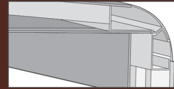
INTERLOCKING CEILING-TO-SIDEWALL CONSTRUCTION helps keep the box square. This assures a proper cabinet fit.
