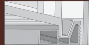
INTERLOCKING FLOOR-TO-SIDEWALL CONSTRUCTION locks tightly to keep out water, dust and noise, and helps eliminate squeaks and rattles.
