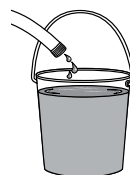
Absorb Charge Water (charger) slows until the bucket (battery) is 90% full.
