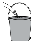
Float Charge Water (charger) slowly trickles into the bucket (battery) until 100% full. Water (charger) will adjust flow to maintain level.
