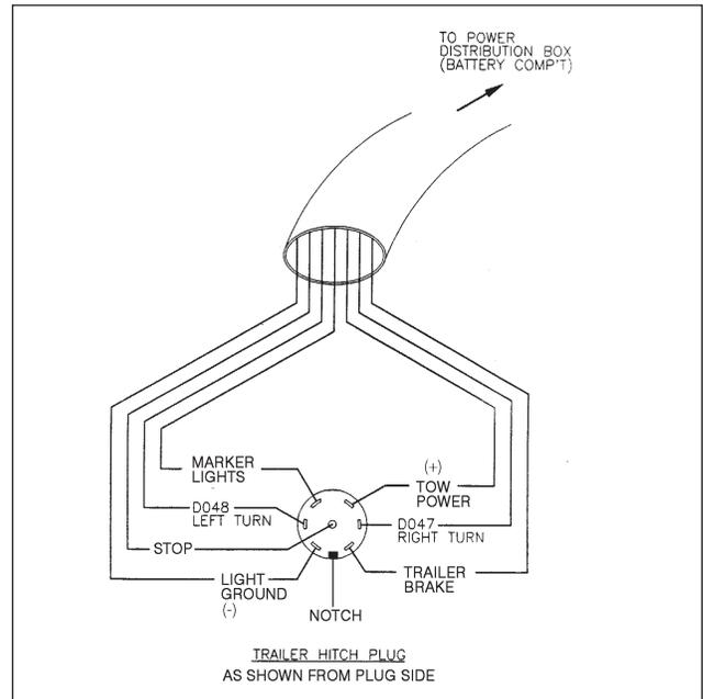
Please note this connector does not provide separate positions for the two turn signals and brake lights. This is necessary for the towed vehicles that do not have separate amber turn signals in addition to the red brake lights.
