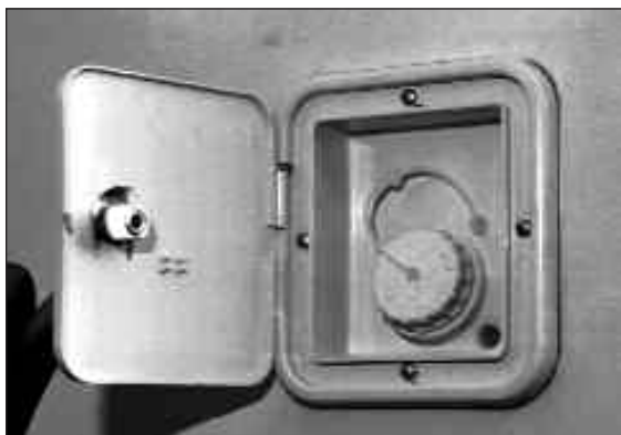
Fresh Water Tank Fill
