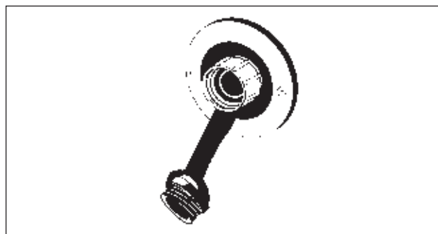
External Fresh Water Connection
