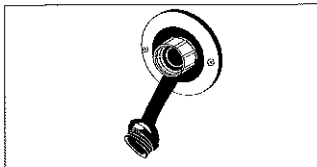
External Fresh Water Connection
