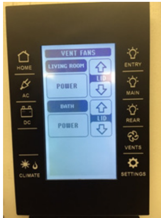
Figure VIII Remote Vent Fan Operating System
