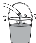
Bulk Charge Water (charger) on full until the bucket (battery) is 80% full.
