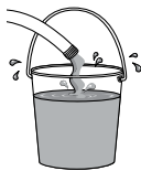
Bulk Charge Water (charger) on full until the bucket (battery) is 80% full.
