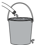
Float Charge Water (charger) slowly trickles into the bucket (battery) until 100% full. Water (charger) will adjust flow to maintain level.
